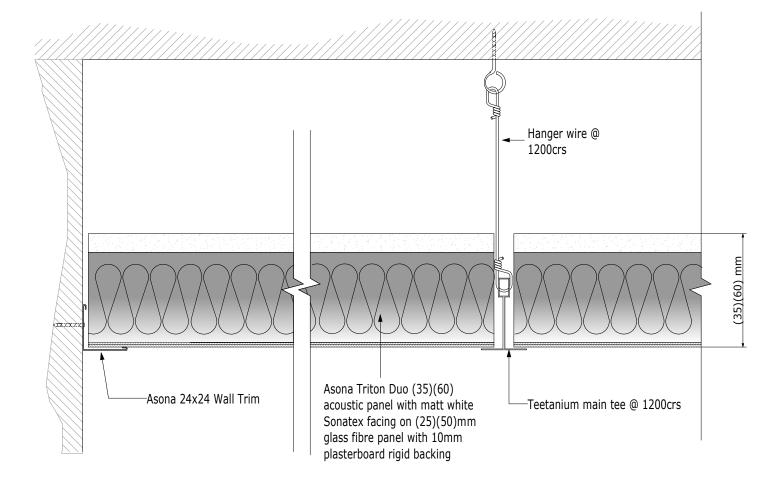
For standard panel dimensions: 600x600x60mm 1200x600x60mm 2400x600x60mm
